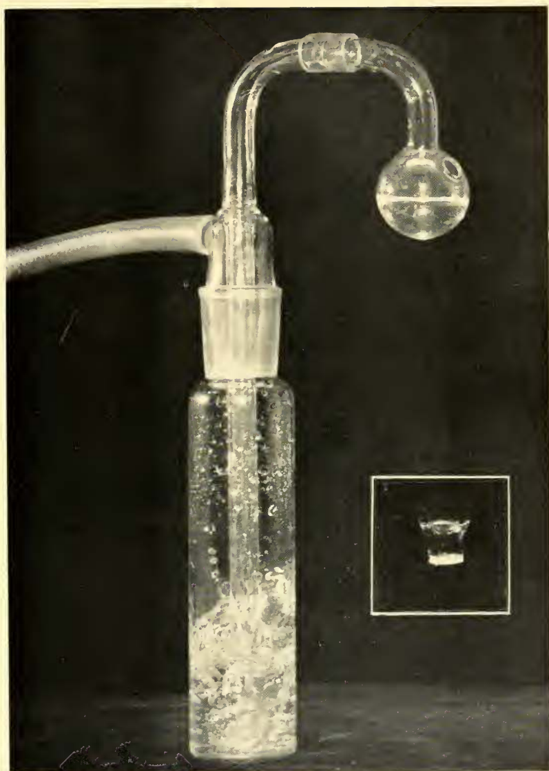
Rosebury-Henderson Capillary Impinger in operation, with air entering first through a May & Druett Pre-impinger. (Inset shows the capillary in still conditions.)
