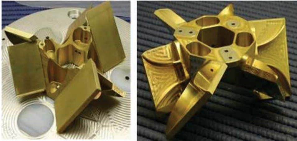
Fig. 10.— Grating Wheel Assembly (Wheel 1).
