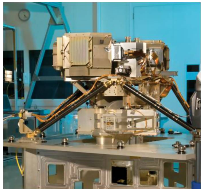
FIG. 1.—The MIRI Flight Model prior to delivery. The optics module structure is aluminum, and it is mounted to JWST with a (black) CFRP hexapod truss. See the electronic edition of the PASP for a color version of this figure.
