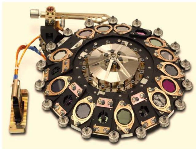
FIG. 9.—The MIRI Filter Wheel Assembly (FWA). See the electronic edition of the PASP for a color version of this figure.
