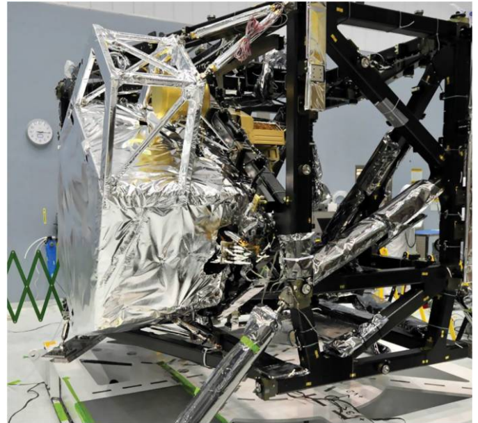
FIG. 5.—MIRI on ISIM and enveloped by the MIRI Thermal Shield, which provides a 23 K radiative environment. See the electronic edition of the PASP for a color version of this figure.
