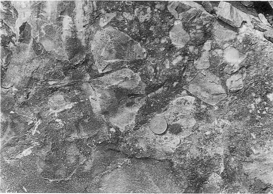
Plate 9: Specimen of agglomeratic tuff from Johore. Trace amounts of fibrous silica detected.
