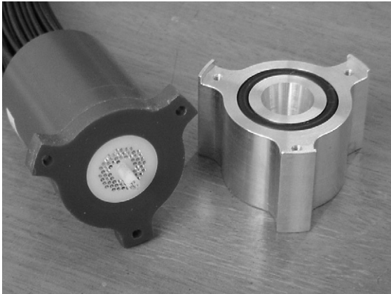
Fig. 13. A collar and cone. The tea-strainer and the central tube holding the PIN photodiode fibres are seen at the front of the collar, and the fibre bundle (ponytail) is emerging from its rear.
