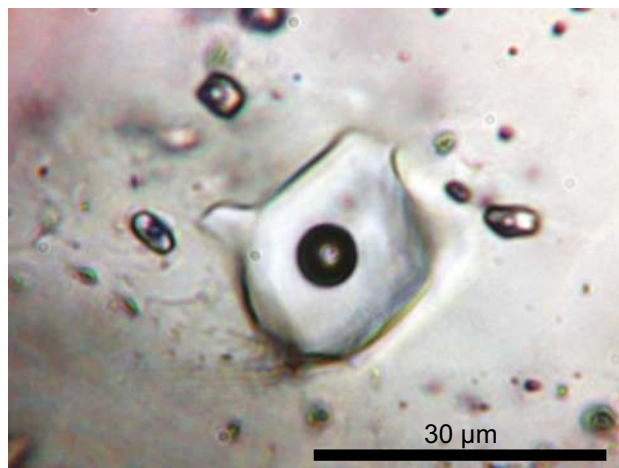
Fig. 3 An isolated melt inclusion (re-homogenized at 700 °C and 3 kbar) in quartz of an aplite from the Königshain granite, see text for details.
