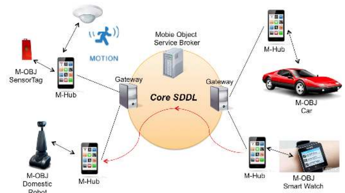
Figure 1. The extended SDDL: M-Hubs are connected both to the SDDL Core and to nearby M-OBJs, for opportunistically transmitting their sensor data and/or remote actuation commands.
