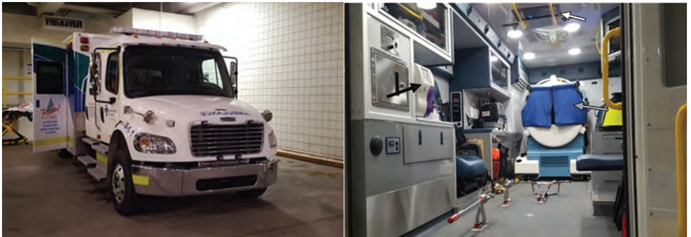
Figure 1: The mobile stroke unit based at the University of Alberta Hospital in Edmonton (left photo). The ambulance (right photo) is equipped with a computed tomography scanner (grey arrow), “point-of care” laboratory (analyzer model pochH-100i, Sysmex Canada; black arrow) and telemedicine equipment (white arrow).
