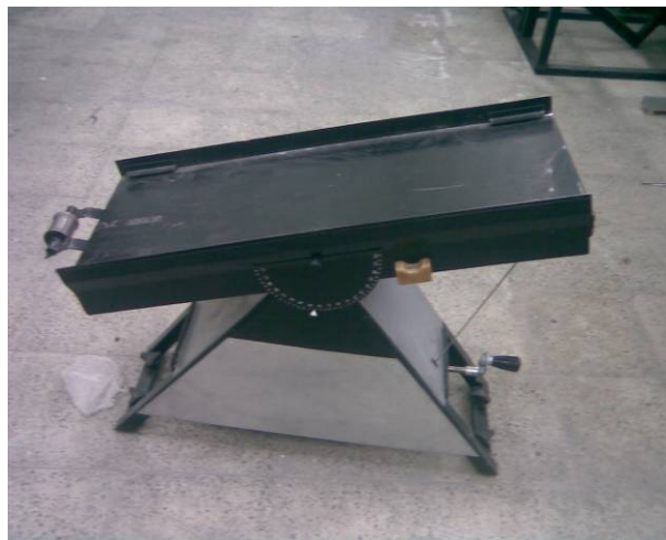
Figure 2. Apparatus to determine coefficient of static friction
