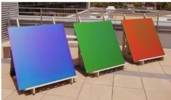
Fig. 13. Demonstrator modules of the format 1.0 \times 1.0 \text{ m}^2 . Slight changes in color close to the edges are caused by deposition rate variations in the lab coater.
