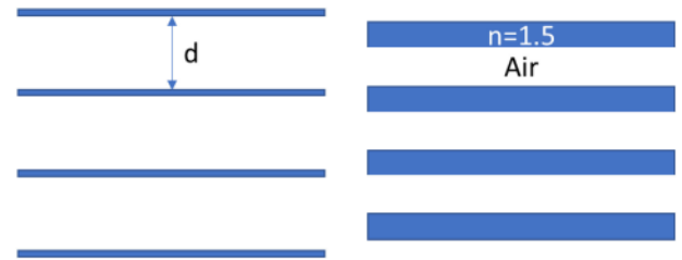
Fig. 3. Left: thin lamella system described by the simple Bragg model. Right: Bragg stack consisting of four layers with defined thickness.
