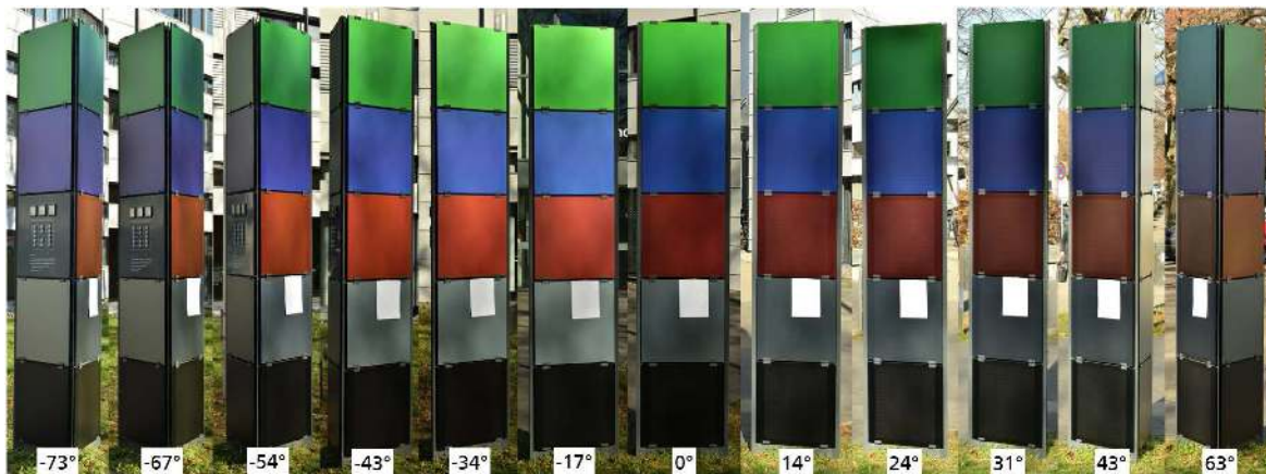
Fig. 12. Series of photographs of the stele with demonstrator modules, taken from 12 different azimuth angles (73° left to 63° right).
