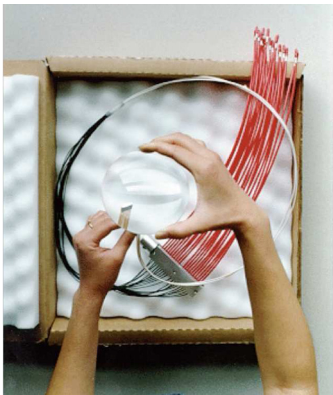
Figure 5. Photograph of an SDSS fiber harness. The ends, which are plugged and unplugged during operations, are protected by tough nylon tubing, which terminates in the anchor block. The lens enlarges the view of the v-groove block termination at the slit end.
