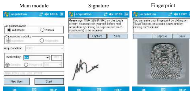
Fig. 7. Screen captures of the main module (left) and the different modules of the DS3 acquisition software for PDA.
