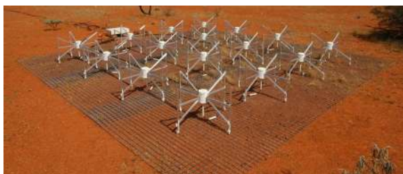
Fig. 2. Photograph of one of the 32 MWA tiles currently deployed at Boolardy, Western Australia. The 5 \times 5 \text{ m}^2 wire mesh ground plane is laid directly on the ground and the dipoles are clipped onto the mesh. The beamformer box is seen in the background.
