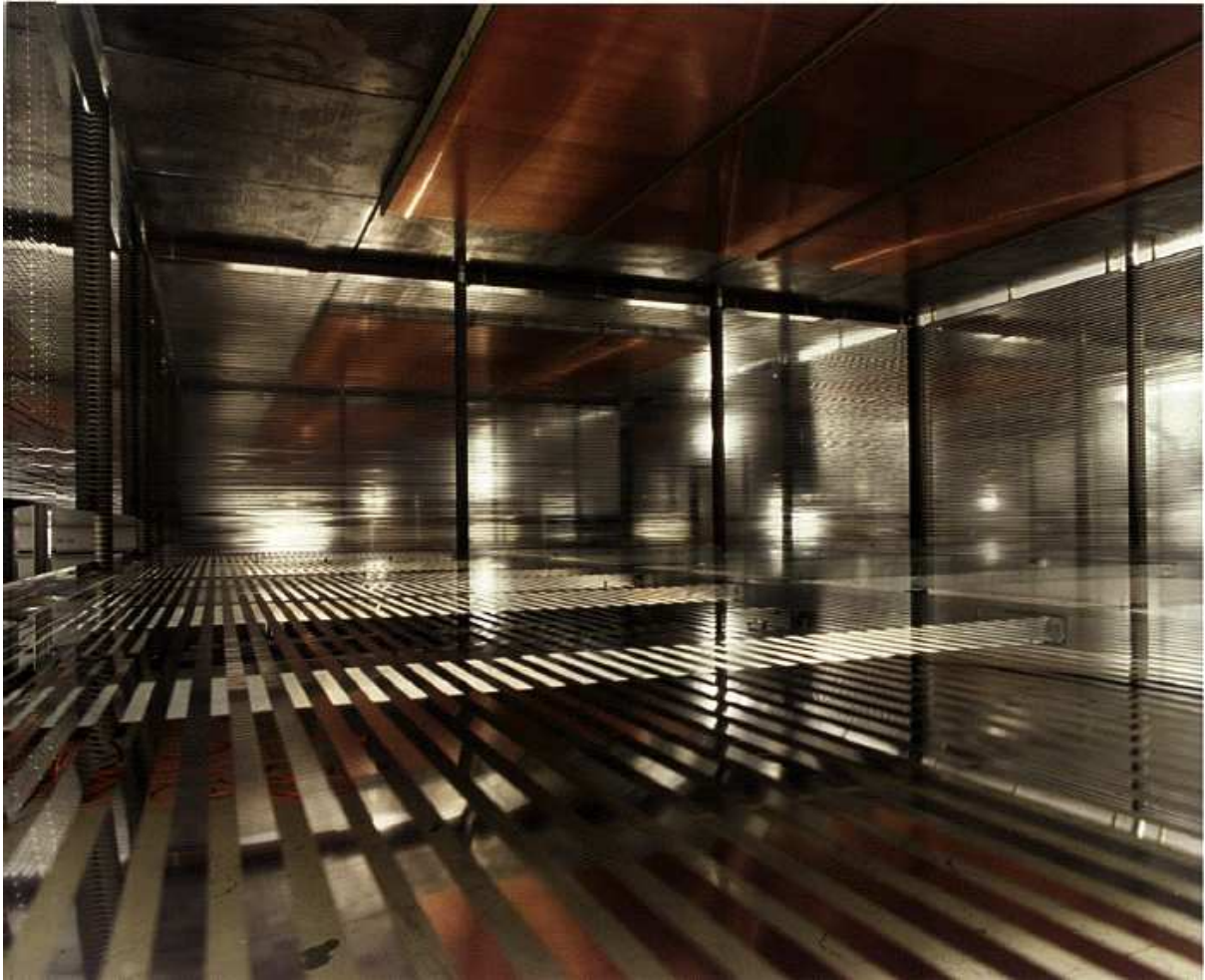
Figure 13: View into the field cage of a MTPC.
