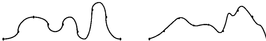
Figure 6.4 Under-sampling. Two different surfaces that produce the same set of sampled height values when sampled at the same locations.
