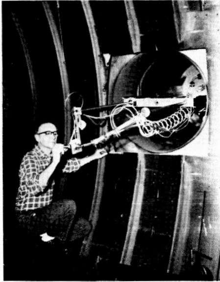
FIGURE 7. - RESISTOJET PLUME CHARACTERIZATIONS. (24)
