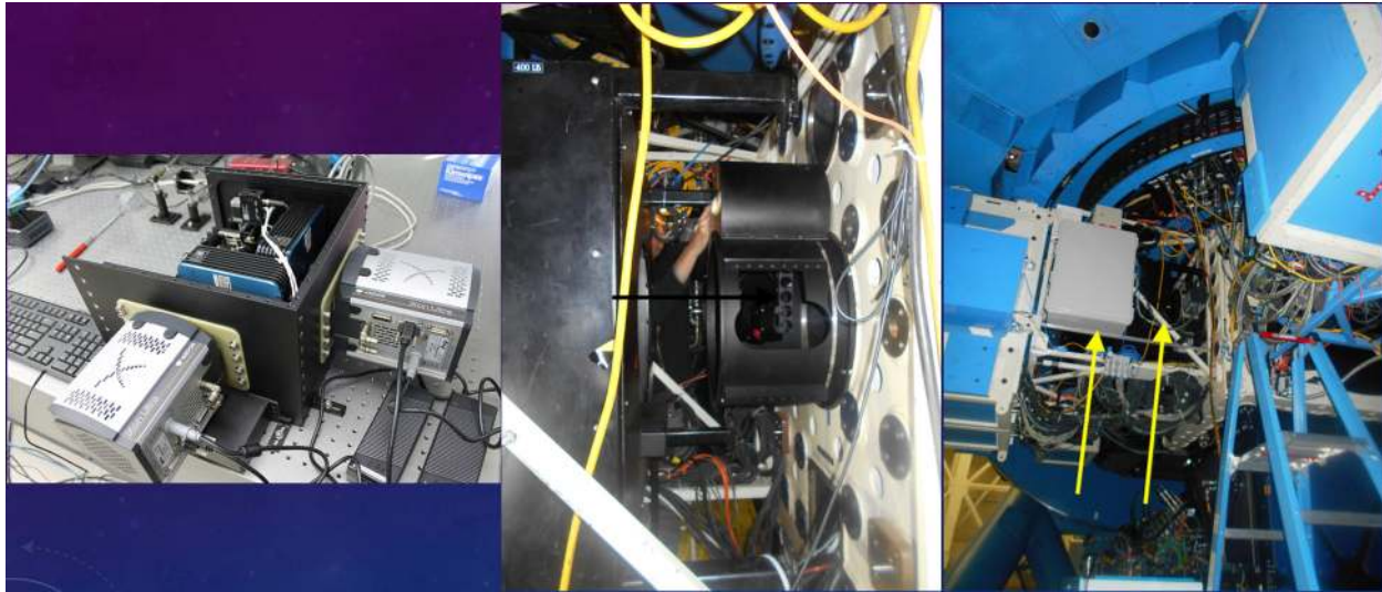
FIGURE 5 | (Left) One of the two identical speckle imagers under construction at the NASA Ames Research Center. The two grey boxes extending out of the black box are the two Andor EMCCD cameras. (Middle) A close-up view of the instrument mounted on Gemini at the GCAL port and (Right) a view of the instrument (black box) with the associated power supply, electronics, and computer unit (white box). See yellow arrows.
