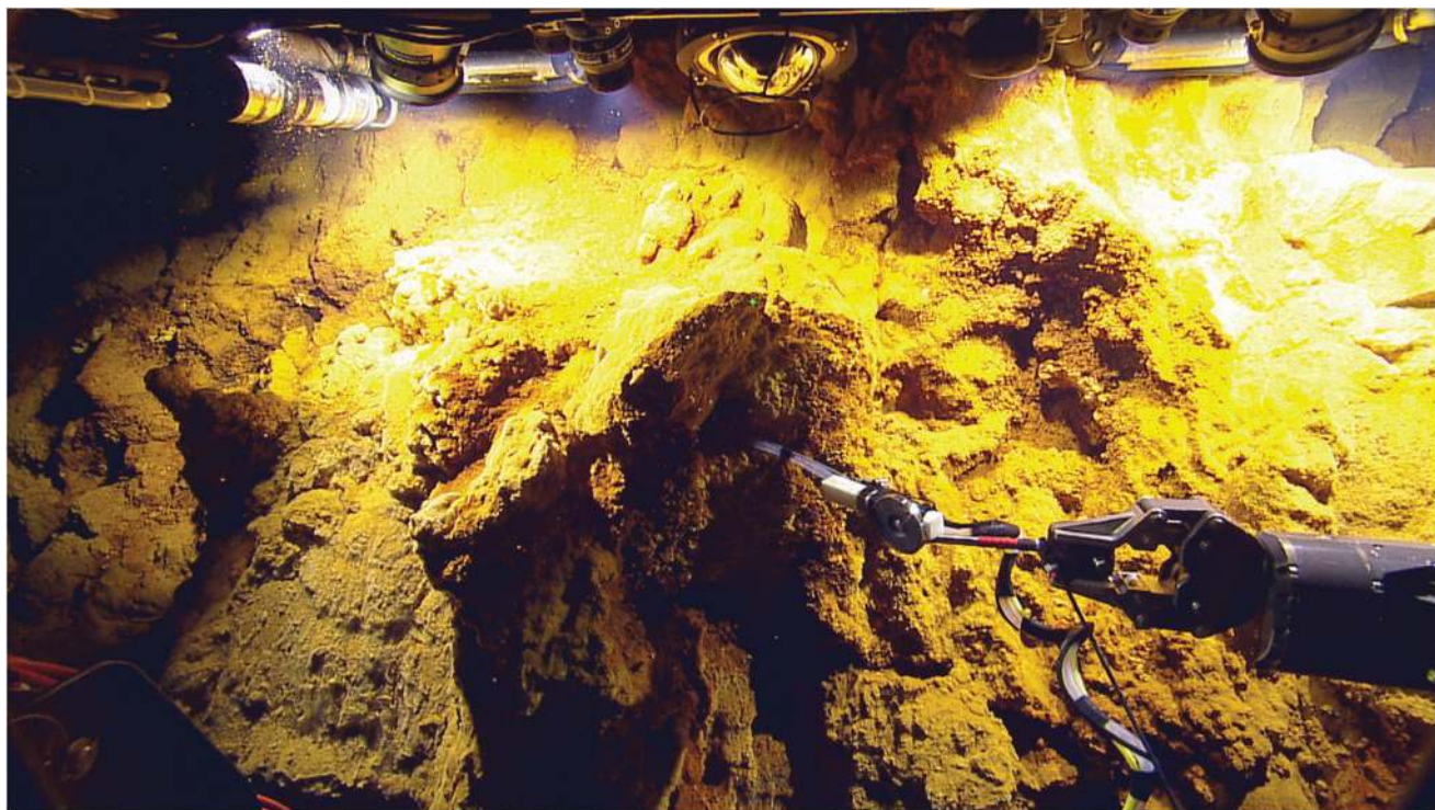
FIG. 4. ROV Hercules sampling for hydrothermal fluid compositions and associated microbiology at the Dragon Cave vent, Loihi seamount, during the SUBSEA program, a model NOAA/NASA co-funded R&A collaboration with dual focus on Ocean Exploration and Ocean World analog studies. Photograph courtesy of Ocean Exploration Trust. R&A, Research and Analysis.
