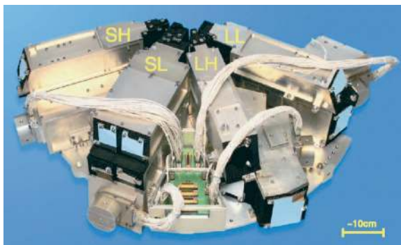
FIG. 22. (Color) The IRS modules, short-high, short-low (which includes the peak-up cameras), long-high, and long-low installed on the multiple instrument chamber test plate before integration into the cryogenic telescope assembly. The location of the spectrograph slits in the focal plane is shown in Fig. 7. Reproduced courtesy of Houck et al. (Ref. 21)
