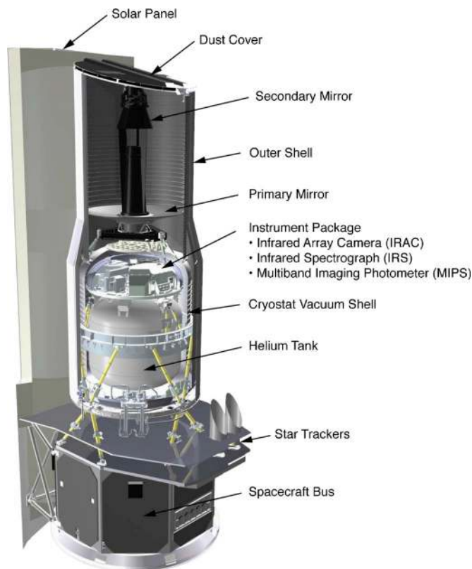
FIG. 6. Cutaway view of the cryogenic telescope assembly showing the details of its mounting to the spacecraft bus (SCB) and internal details of the structure. Kinematic, conductive isolation from the SCB is accomplished using gamma-alumina bipod struts (yellow). The titanium bipod flexures that attach the cryogenic telescope bulkhead to the cryostat and the primary mirror to the bulkhead are clearly visible in this view, as is the attachment point of the metering tower adapter ring to the bulkhead. Courtesy of Ball Aerospace.
