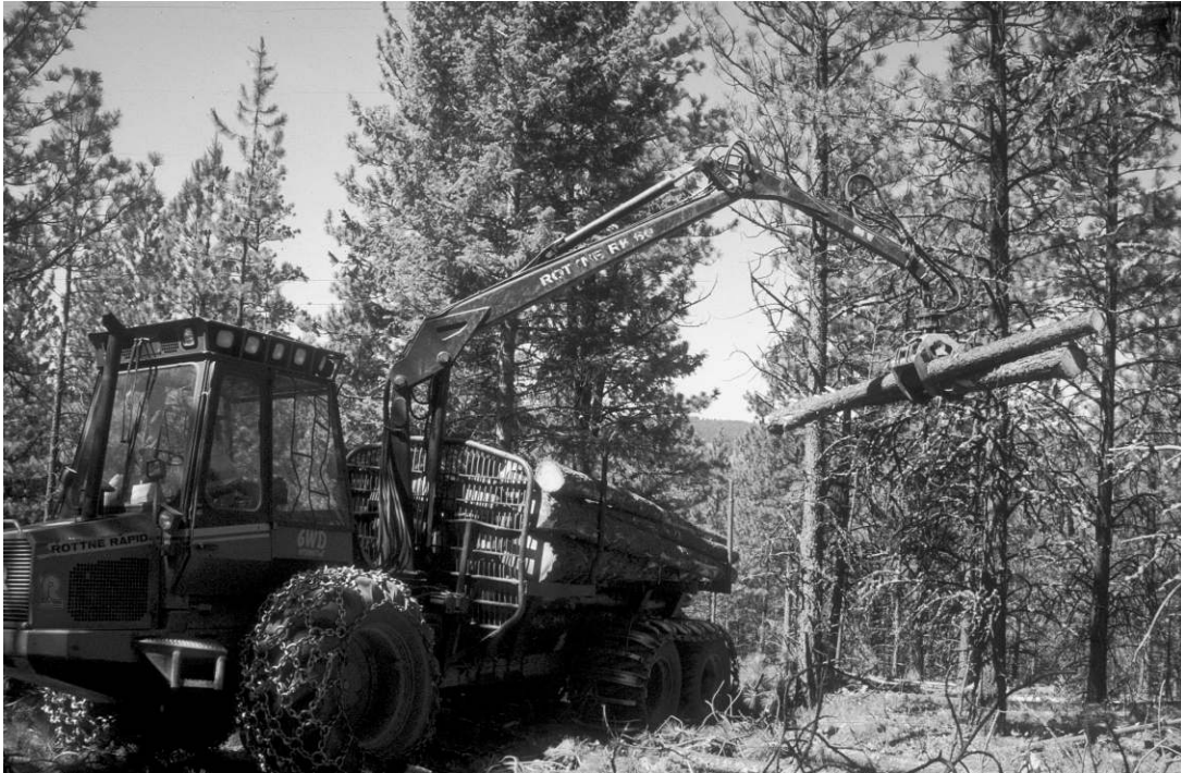
PLATE 1. Treatments in the national Fire and Fire Surrogate study involved under-burning and some form of mechanical fuel reduction, such as this forwarder working with a single-grip harvester to remove small-diameter ponderosa pine at the northeastern Oregon study site. Photo credit: A. Youngblood.
