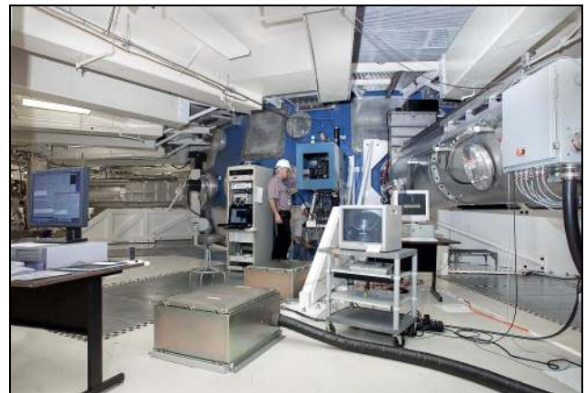
Fig. 6. View of NIF Target Chamber at the equator level. Visible in this photograph are target positioning and alignment systems.
