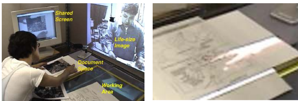
Figure 3. The configuration of the Agora system for the experiment. Details of objects can be referred to in different ways through the different spaces. The image on the left shows the different spaces of Agora. A large life sized image provides access to the remote participant. A working area projects a general view of the remote desktop. Details can be discussed when documents are placed in a 'document space'. When a remote participant gestures over the document space of shared screen their conduct is projected over the 'real' physical object in the local domain. On the right is detail showing how a remote participant's projected hand appear to the local participant.
