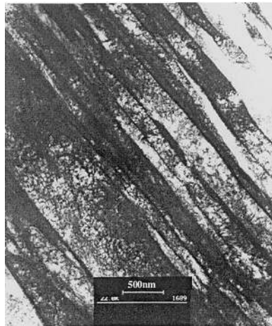
Fig. 2. Transmission electron micrograph of the interior of a block in lath martensitic steel. The bright-field micrograph shows a refined, sub-micron lath size. The diffraction pattern shows the laths are crystallographically almost identical, that is, they behave as a single crystal.
