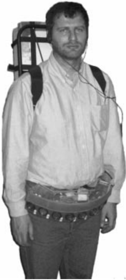
Fig. 2. The NavBelt prototype.
