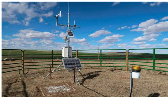
FIG. 3. Station photo illustrating tripod configuration, equipment, and cattle panel configuration at the Arthur 8S Nebraska Mesonet site. The photo was taken at the conclusion of annual maintenance on 16 Jun 2017.
