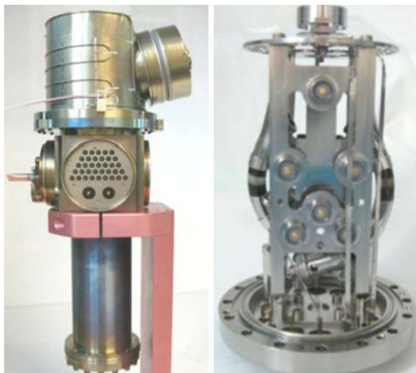
Fig. 8 The mass spectrometer housing is shown in the left panel and the detector assembly on the right . The outside diameter of the detector housing is 5.08 cm. The larger pins on the welded electrical feedthrough assembly are for the RF voltages applied to the quadrupole rods. The pinch-off tube is seen to the left of the feedthrough assembly. The dual detector assembly shown at right is mounted on a flange that utilizes a gold plated Inconel “c” seal to achieve ultra-high-vacuum. The NMS specifications are shown in Table 1
