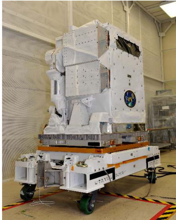
Figure 2. The NICER flight payload in a nearly fully integrated configuration, blanketed and stowed against the flight A-FRAM plate.
