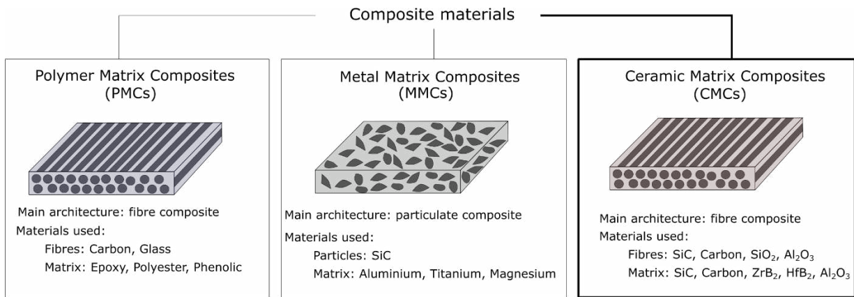
Figure 1 Classification of the composite materials depending on the nature of the matrix showing for each of them the main reinforcing architectures and materials used.
