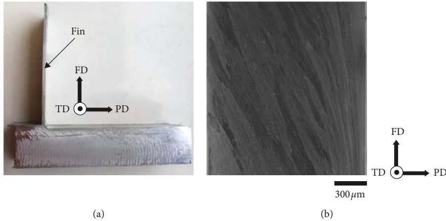
FIGURE 3: (a) A sample after PFM processing. (b) SEM microstructure across the thickness of the fin for the case of t = 0.75 .
