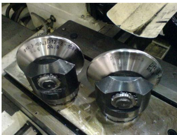
Fig. 6. Roller burnishing thrust pulleys
