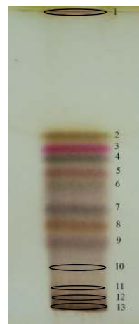
FIGURE 1: 1D separation of Juniperi Oleum compounds. The mobile phase: toluene and ethyl acetate (94 : 6 v/v). The zones were derivatized with the anise aldehyde-sulphuric (VI) acid reagent.
