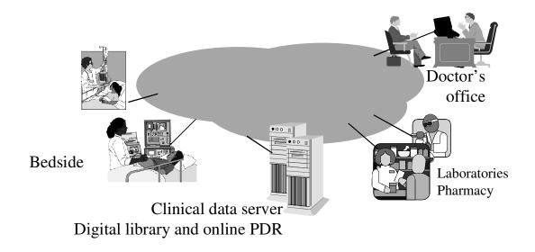
Figure 1: Although one thinks of a hospital network as being a single system, such a network actually superimposes one or more critical care networks on a clinical database network.
