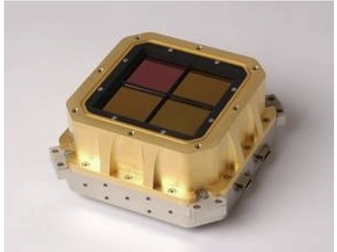
Figure 1. Illustration of the 2 \times 2 mosaic WIRCam detector array. Each chip features a HAWAII-2RG near-IR detector with 18 \mu\text{m} pixels. The patrol field has 2040 \times 2040 active pixels with a 4 pixel wide border of reference pixels per chip. The field of view of the full detector array is about 21' \times 21' with 45'' wide interchip gaps. Image courtesy of Academia Sinica Institute of Astronomy and Astrophysics (ASIAA).
