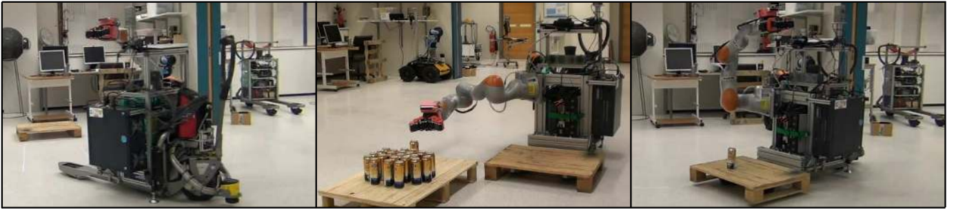
Fig. 6. Testing : (Left) The robot picks up an empty pallet in a designated zone; (Middle) The robot navigates to a loading zone where a can is detected and picked up; (Right) The loaded pallet is transported to a target location (see the video attachment to this article).
