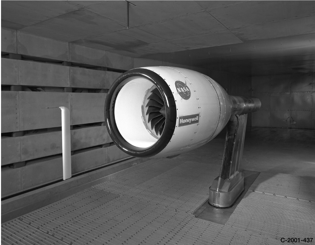
Figure 4.—Quiet high speed fan in test section.
