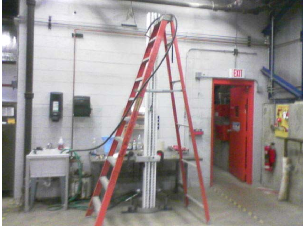
Fig. 17.83: Photograph of the 7-layer X-Y prototype used to measure transmission of swelling from hydrostatic pressure.
