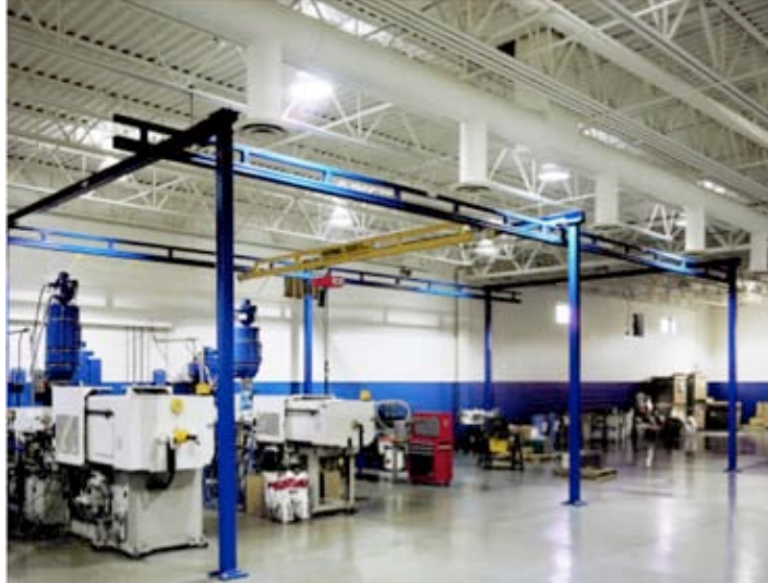
Fig. 13.38: Commercially available free-standing crane of the type to be used in the module assembly.
