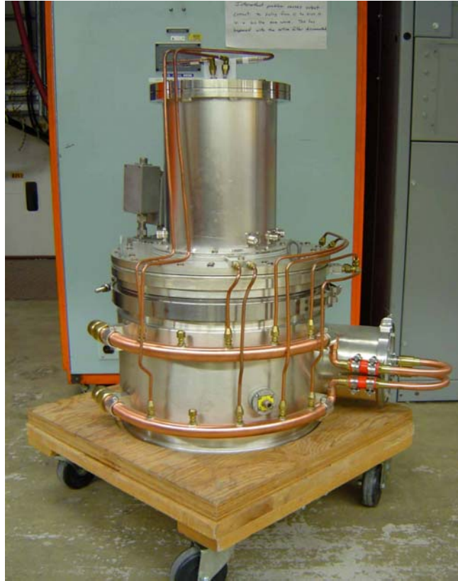
Fig 8.20: Picture of the power tube assembly. We can see the matching section on top and the copper cooling lines. The power tube is located at the bottom of the assembly.
