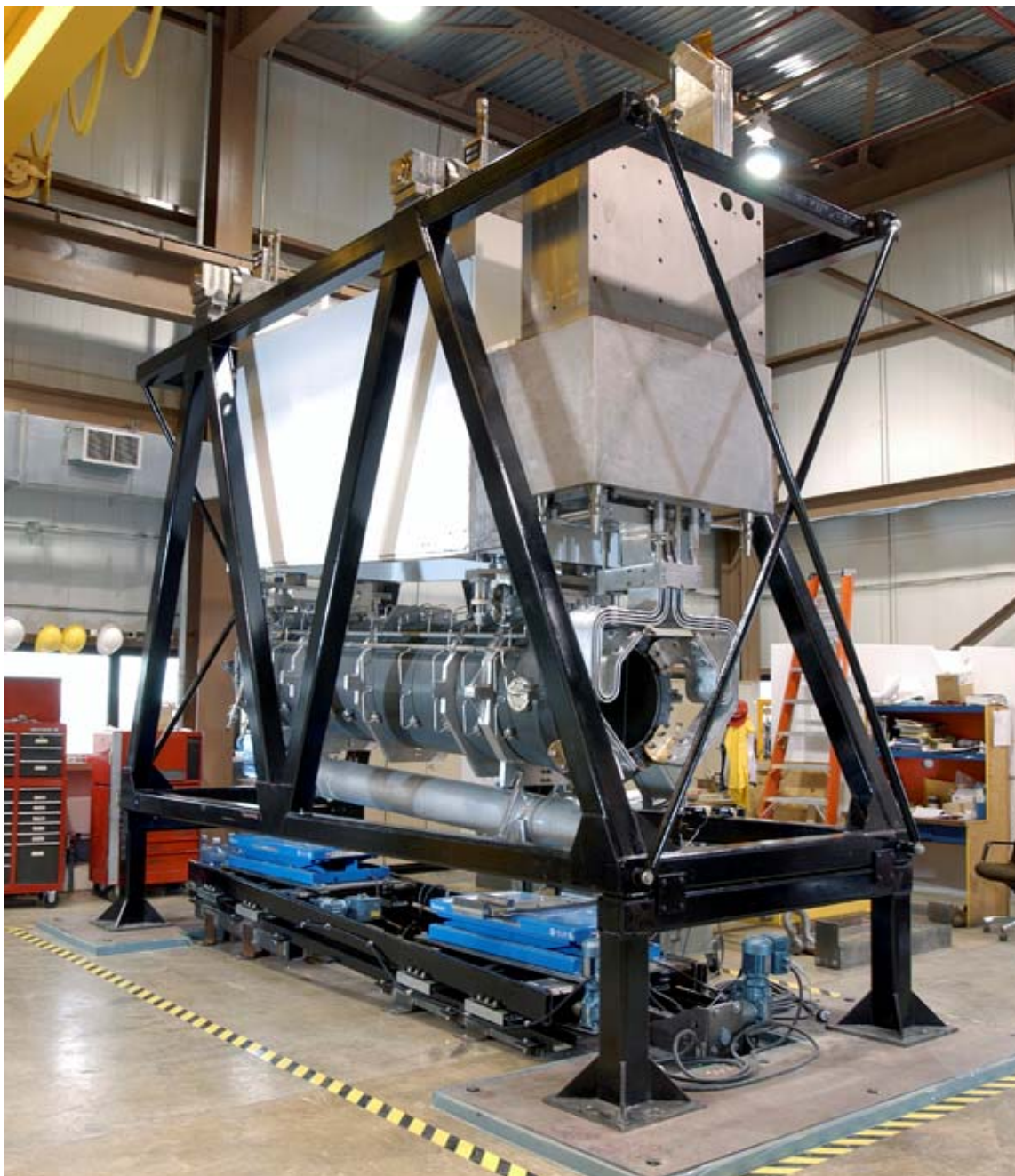
Fig 8.44: Horn 2 attached to module in the MI-65 service building.
