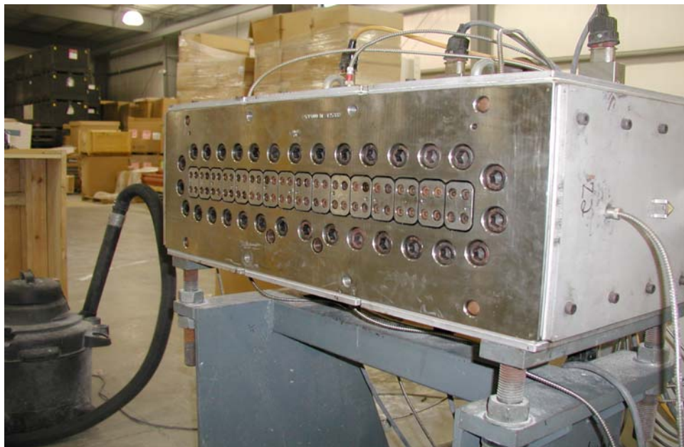
Fig. 12.5: The custom NOVA prototype 16-cell die. PVC resin moves right to left and exits the die through the scalloped profile shown in this view.
