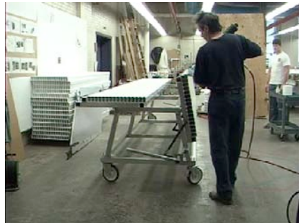
Fig. 13.39: Table used to glue two 16-cell extrusions into a 32-cell extrusion assembly. The 2 extrusions are shown in white on the drawing.
