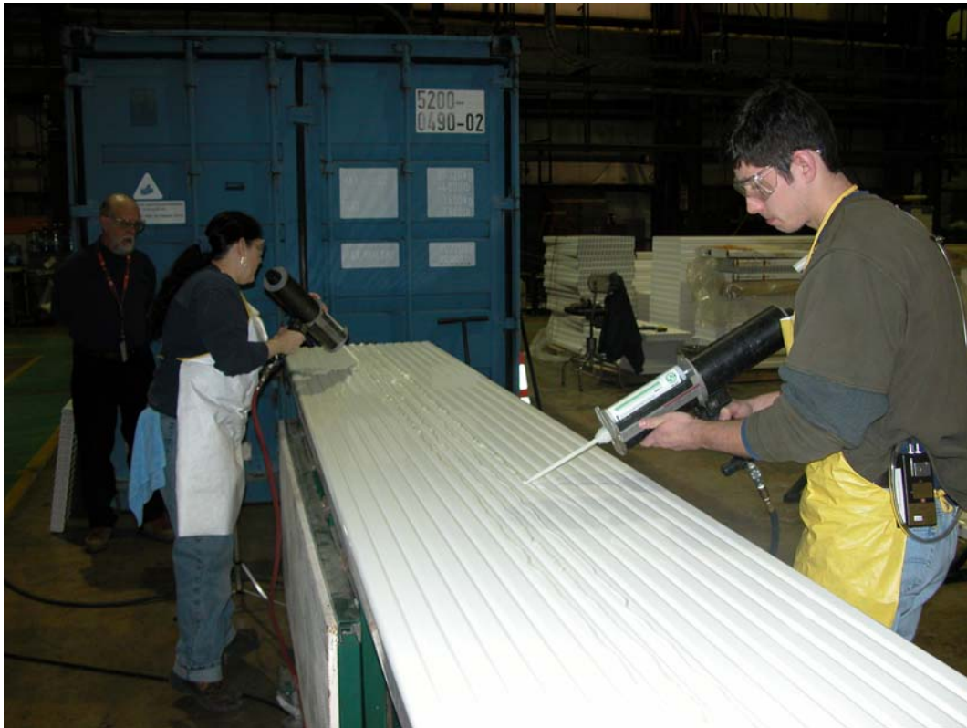
Figure 17.92: Applying the adhesive.
