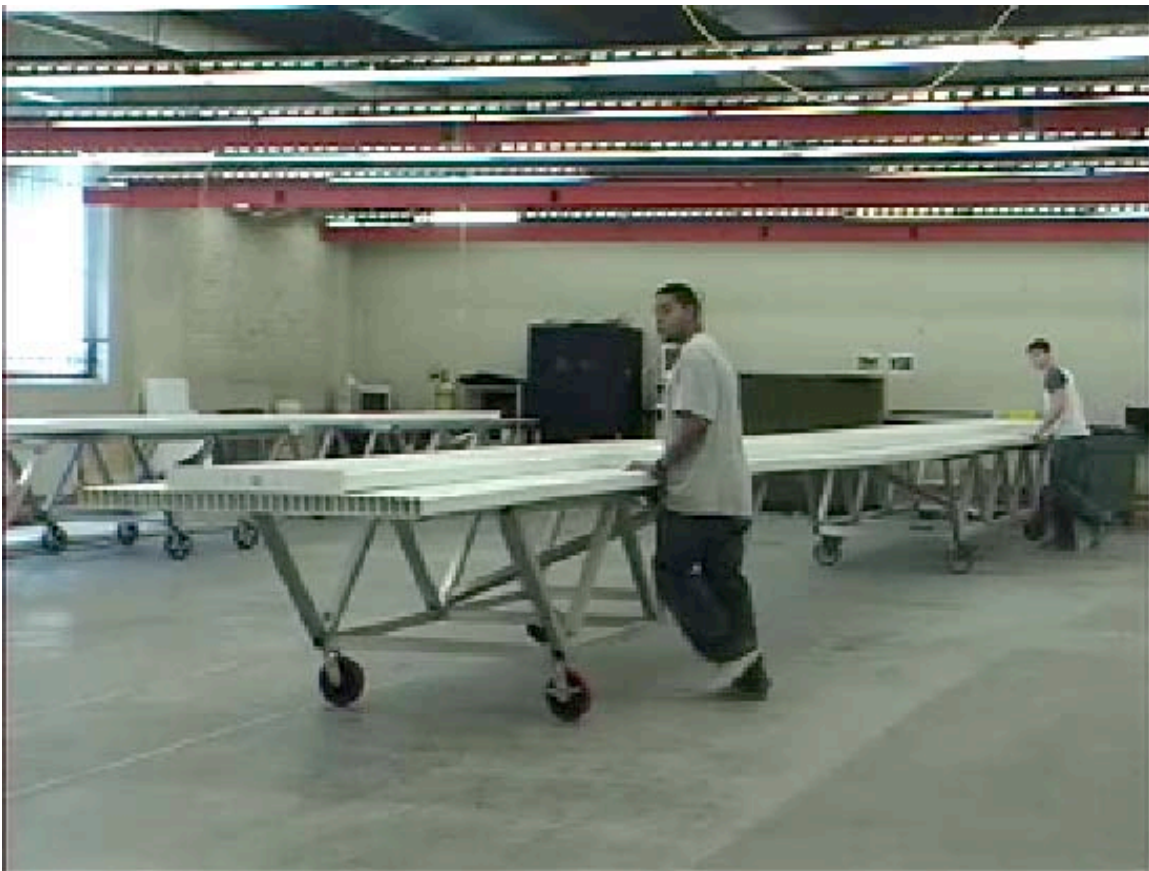
Fig. 13.44: Rolling a work table with an extrusion assembly.
