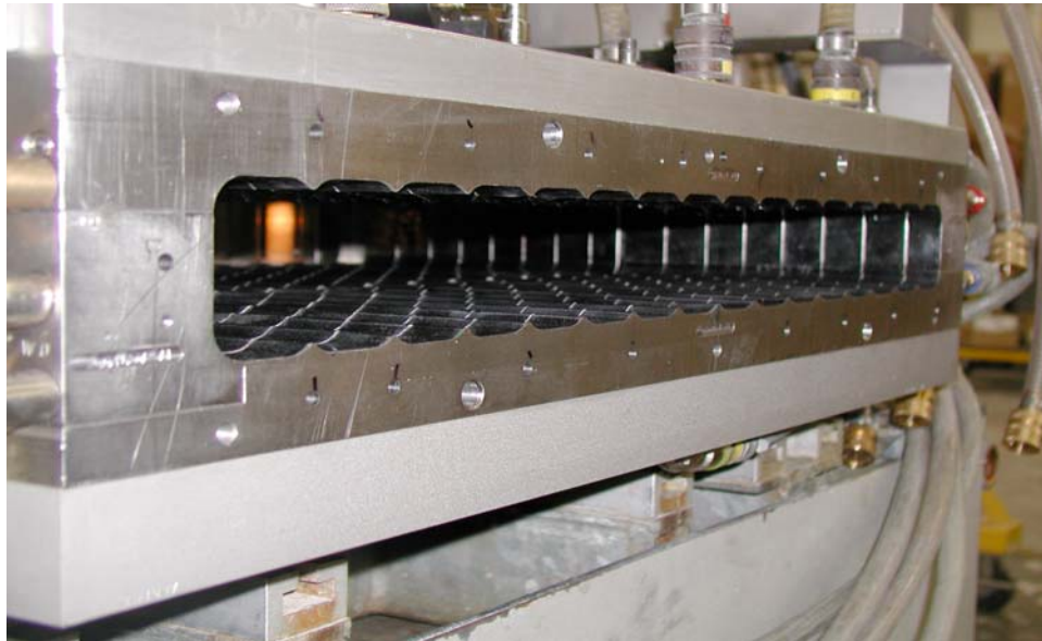
Fig. 12.6: The custom NOVA vacuum sizing tool. During production, this tool is in close proximity to the exit face of the die. As the molten PVC exits the die the water-cooled sizing tool keeps extrusion shape from collapsing by sucking the outside walls of the extrusion against the walls of the sizing tool .
