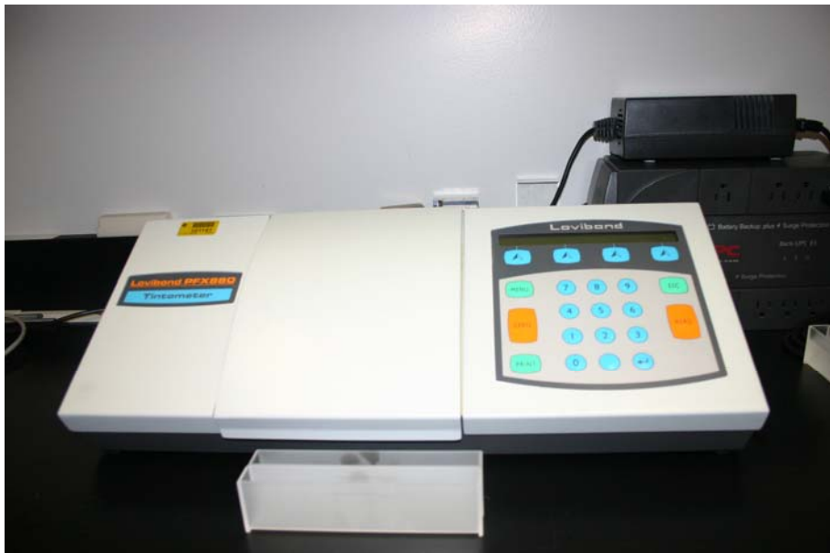
Fig. 10.14: The Lovibond PFX880 Tintometer in the Indiana University lab. In the foreground are 6" optical glass cells.
