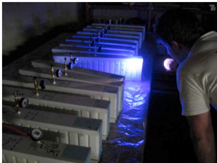
Fig. 13.33: Inspecting the test joints for the fluorescence that would indicate a leak
