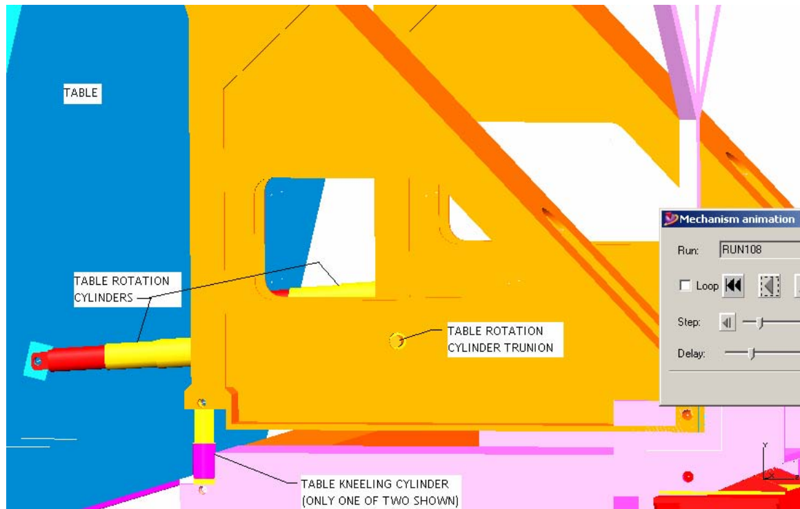
Fig. 17.138: Detail of the block pivoter showing the table approaching vertical, highlighting the table rotation cylinders and one table kneeling cylinder.
