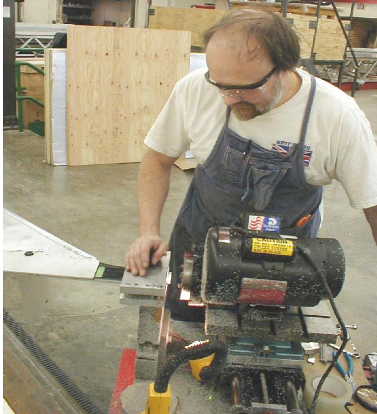
Fig. 13.55. Flycutting an optical connector.
