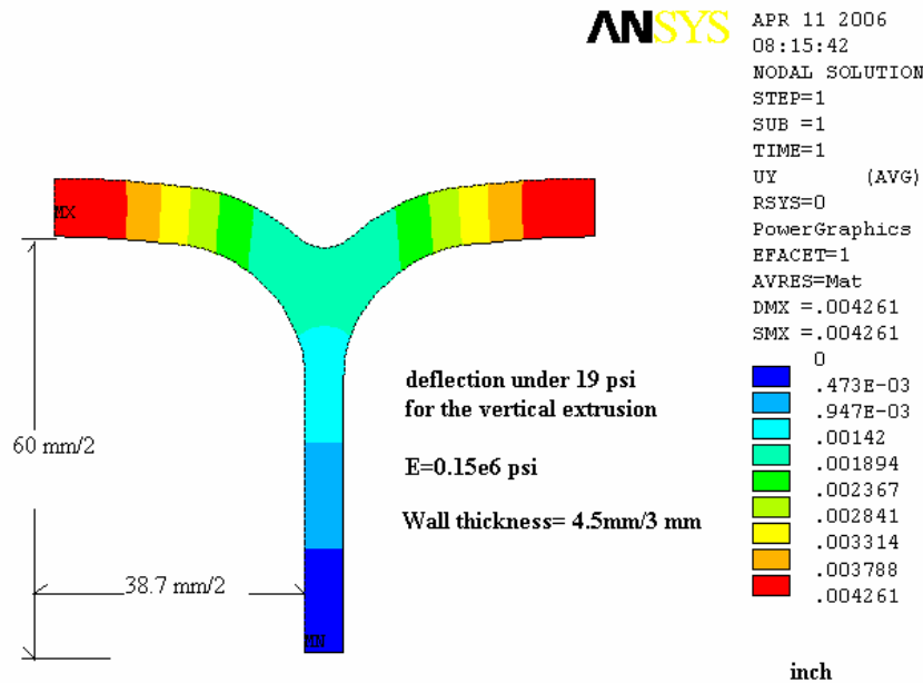
Fig. 17.7: Stress distribution for one vertical extrusion cell subjected to 19 psi with E = 150 ksi.
