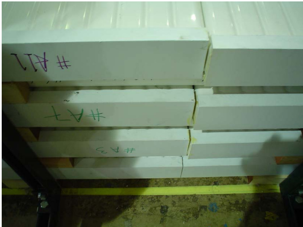
Fig. 17.113: Misalignment of end seals and gaps between vertical end seals and horizontal extrusions in IPND 8-plane prototype.
