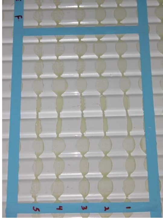
Fig. 17.98: Compression along boundary between adjoining extrusions.
