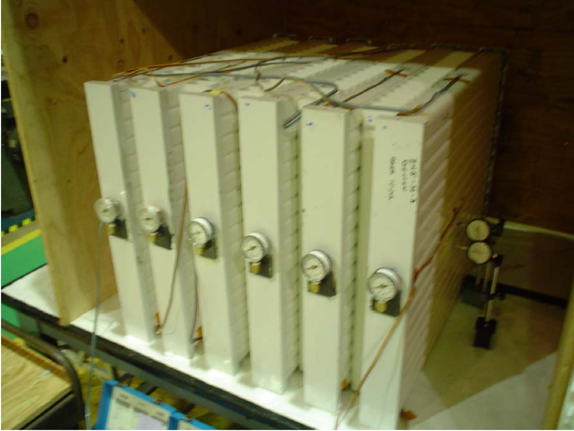
Fig. 17.89: Photograph of the 11-layer prototype showing dial indicators (to measure PVC deformation) and strain gauges.
