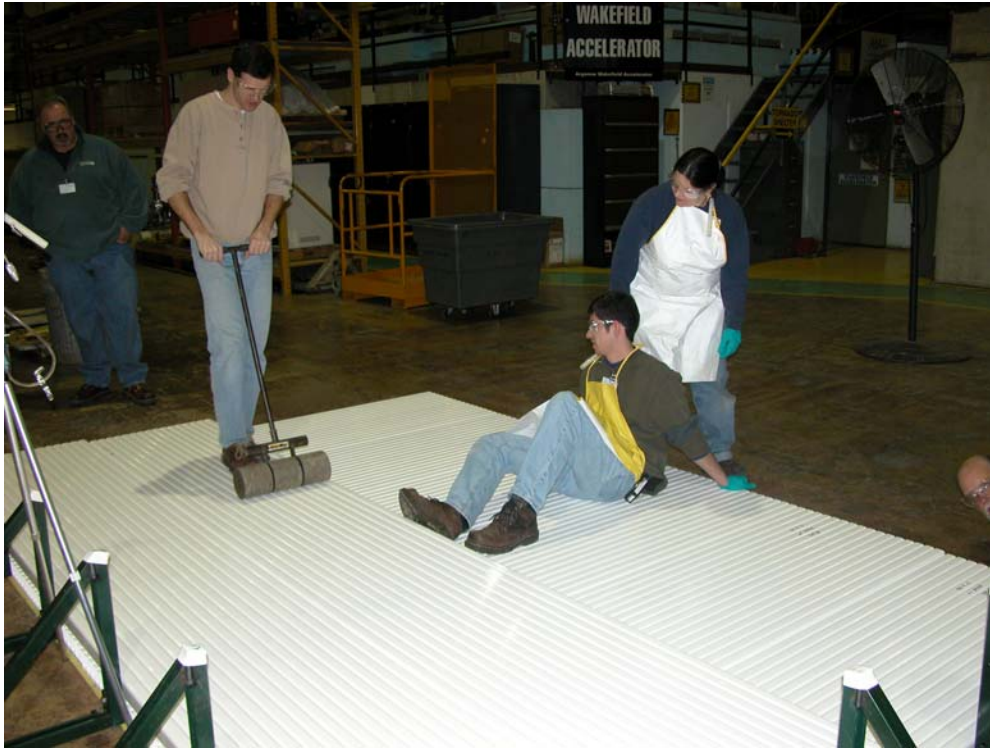
Fig. 17.93: Rolling the extrusion and applying pressure to remove the banana shape.
