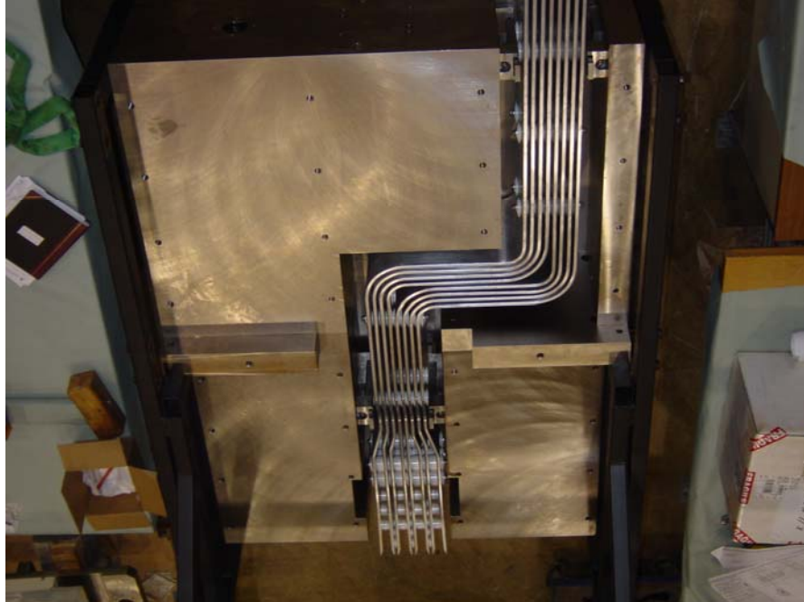
Fig 8.48: Stripline Block Assembly showing labyrinth with the cover removed.
