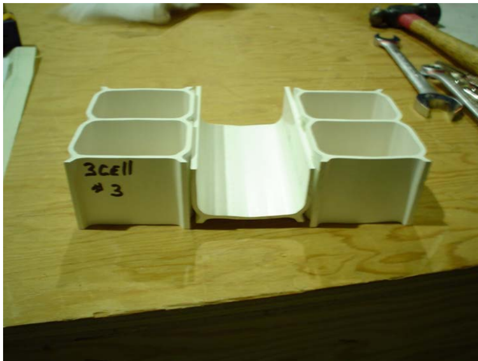
Fig. 17.106: Extrusion assembly used for the shear strength measurement.
