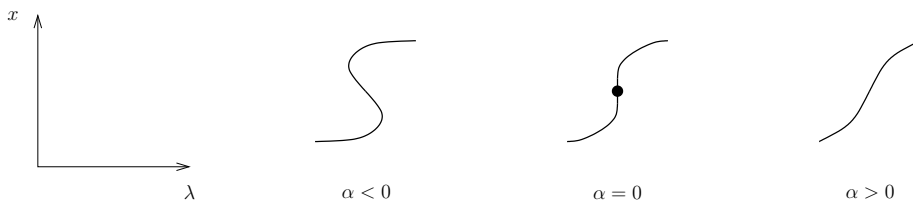
Fig. 2. Solution diagrams for f(x, \lambda, \alpha) = x^3 + \alpha x - \lambda = 0 . The hysteresis point is destroyed for \alpha \neq 0 and there are no singular points for \alpha > 0
