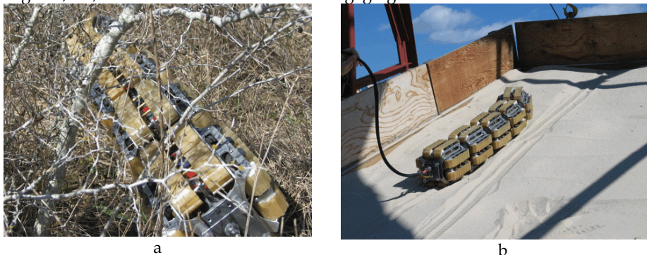
Fig. 11. The OT-8 outperformed the OT-4 on difficult natural terrains, mostly because of the OT-8 larger track sprocket diameter. a - The OT-8 literally plowed through SwRI's underbrush test area, aided, in part, by its more massive weight and greater power. b- Unaffected by sand, the OT-8 had enough power and traction to drive up a 15° inclined bed of deep sand.
