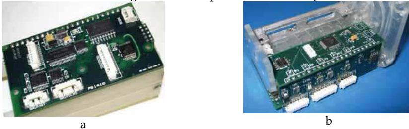
Fig. 18. Electronic control circuit boards in the OT-4.
