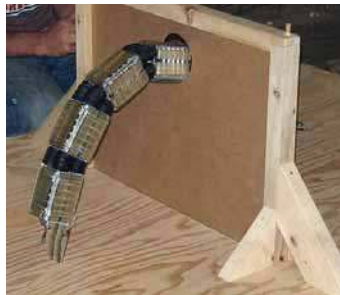
Fig. 6. OT-4 passes through a 10-cm (4") diameter hole, high above ground. Extendable "flipper tracks" in the distal segments allows the robot to straddle the hole without having to support its weight on the sharp edges of the hole in this test at SwRI.
