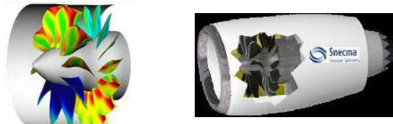
Counter rotating fan with 10 + 14 blades
