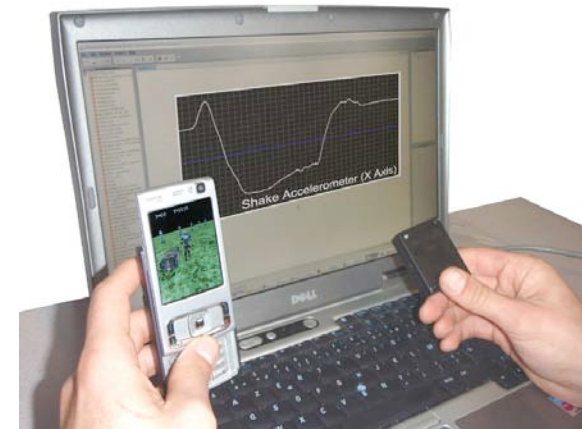
Figure 4. 3D Game on mobile phone with the Shake and oscilloscope visualization tool.
