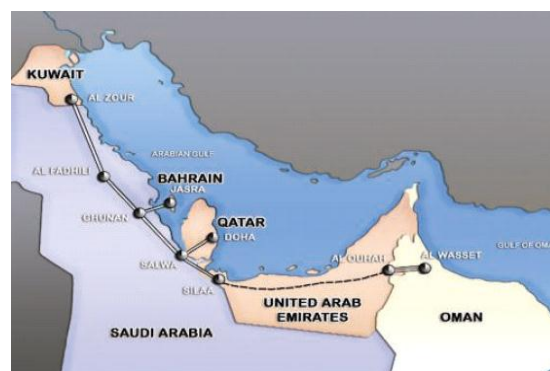
Figure 1. The geographical routes and layout of the GCC interconnection
