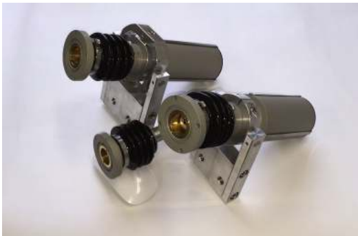
Figure 4: Two mounting points including the actuators with a single and a double gimbal, and a fixed support Figure 5: the pads glued on the back side of the mirror for the fixation to the mounting points
