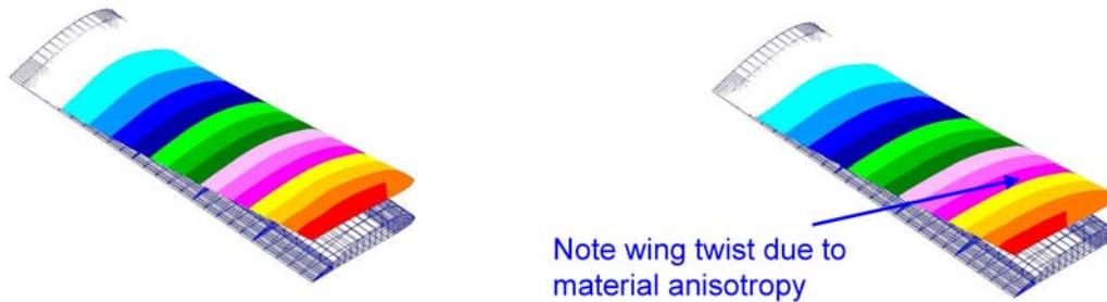
Figure 6: The deformation for the optimum wing designs, without (left) and with (right) aerodynamic constraints
