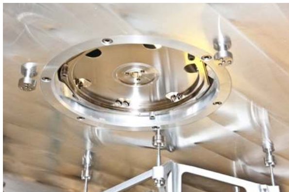
Figure 5: The membrane mounting into the dummy mirror segment.
