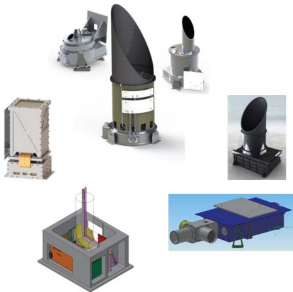
Figure 8. OSIRIS-REx instruments (clockwise from top): OCAMS camera imaging system, OTES thermal emission spectrometer, OVIRS optical and near IR spectrometer, OLA imaging lidar, and the REXIS X-Ray emission spectrometer. Gravity field Doppler observations are obtained with the Deep Space Network (not pictured.)
