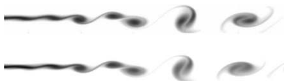
Fig. 3 Instantaneous snapshots of spanwise vorticity distribution: results from [8] (top) and current DNS (bottom)
