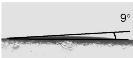
Fig. 12. A water drop on the surface of the ARC with a contact angle of 9°. (Image courtesy of TWI).
