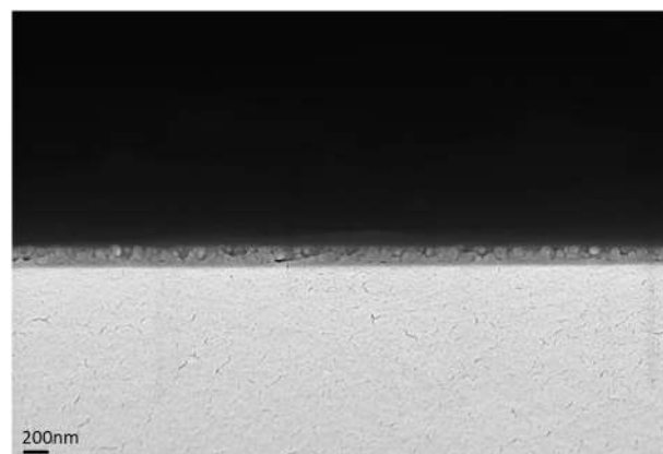
Fig. 4. An SEM image of a cross section of the ARC on a soda-lime glass substrate.
