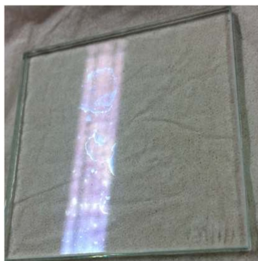
Fig. 11. Optical image of a sol gel coated glass surface showing signs of water damage after 1000 h of DH exposure. (Image courtesy of TWI).
