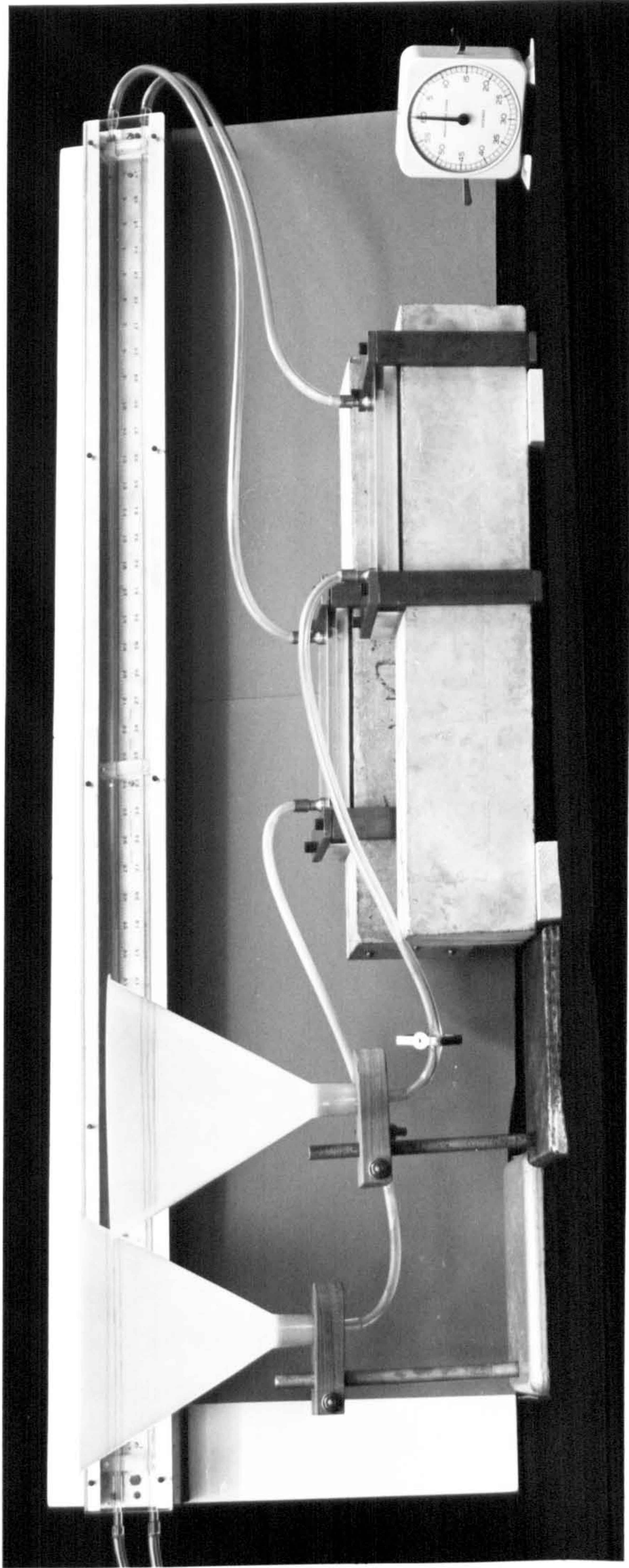
Figure 8.1 : ISAT rigs in operation.
