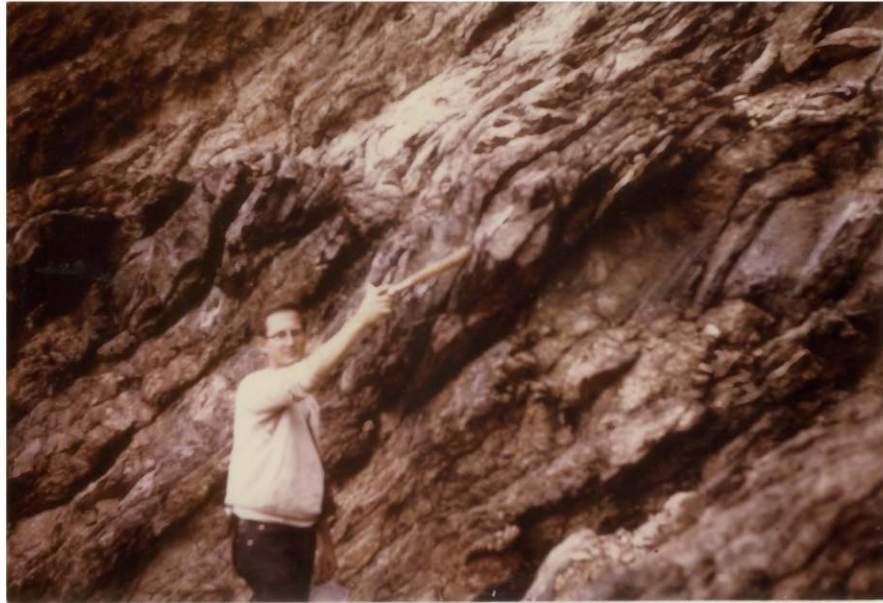
Plate 7. Shearing and mylonitization caused the dark vein indicated. (In the vicinity of LC8-4).
