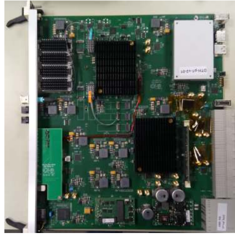
Figure 3. Left: block diagram of the DTH board. Right: DTH P1-v2 board prototype. This prototype uses two KU15P FPGA. The prototype 2 of the board, currently being designed, will use a VU35P FPGA with on-chip HBM.
